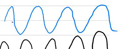
$$V_+(x) + V_-(x) = 2\cos(\delta x) \sin(kx)$$
